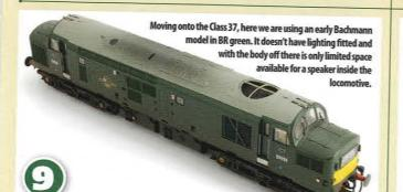
The only space which is available is to roof mount the speaker underneath the fan grille. This does mean sealing the front and rear of the speaker fully and mounting the decoder board to the roof to ensure everything will fit inside. We had already noved the fan moulding from this model prior to starting the sound installation
