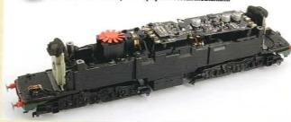
Removing the roo fan opens up a perfect position for a speaker. All that is required to take it out is the release of four small crosshead screws and cutting of the drive band.
