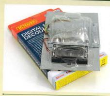
Track Sound (TTS) decoders are supplied with a speaker pre-attached as well as a full manual and suggestions for their installation. The first decoder we are going to work with is the Class 31.
